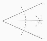
Figure 5: Construction of angle bisector
